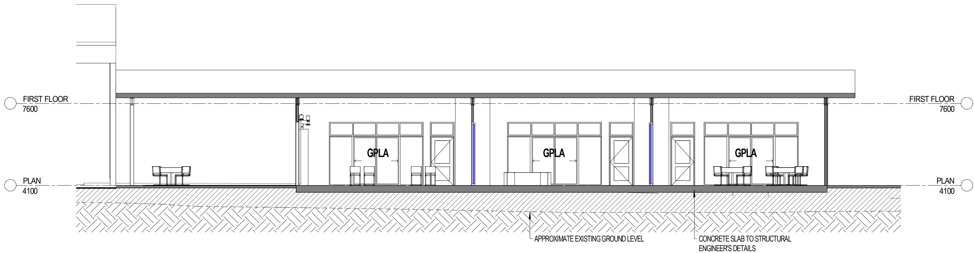
NEW PDHPE BUILDING 1 SECTION BB SCALE: 1 : 100
